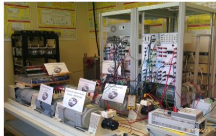
HIL simulation of the 3008 HY4 traction system (« ev » platform)
