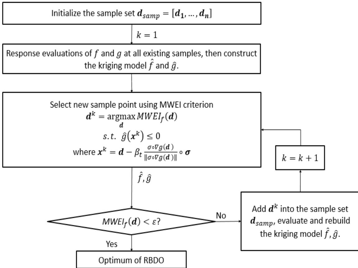
Fig. 2.18. The process of infill strategy with SLA
