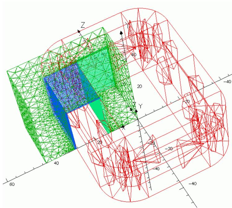
Fig. 3.5. Mesh of 3D FEA for the transformer
