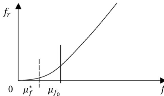
Fig. 1.25. Robust objective function for a smaller-the-better type characteristic (Bhamare et al., 2009)
