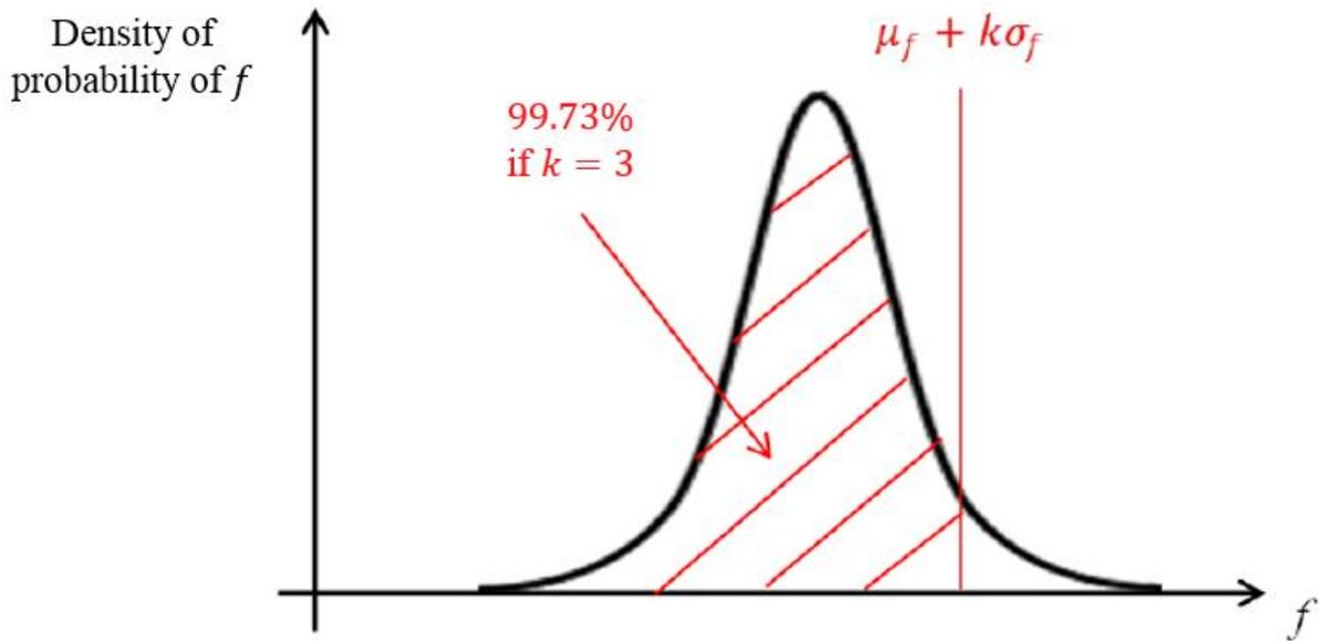
Fig. 1.8. Principe of  $\mu_f + k\sigma_f$  (Picheral, 2013)
