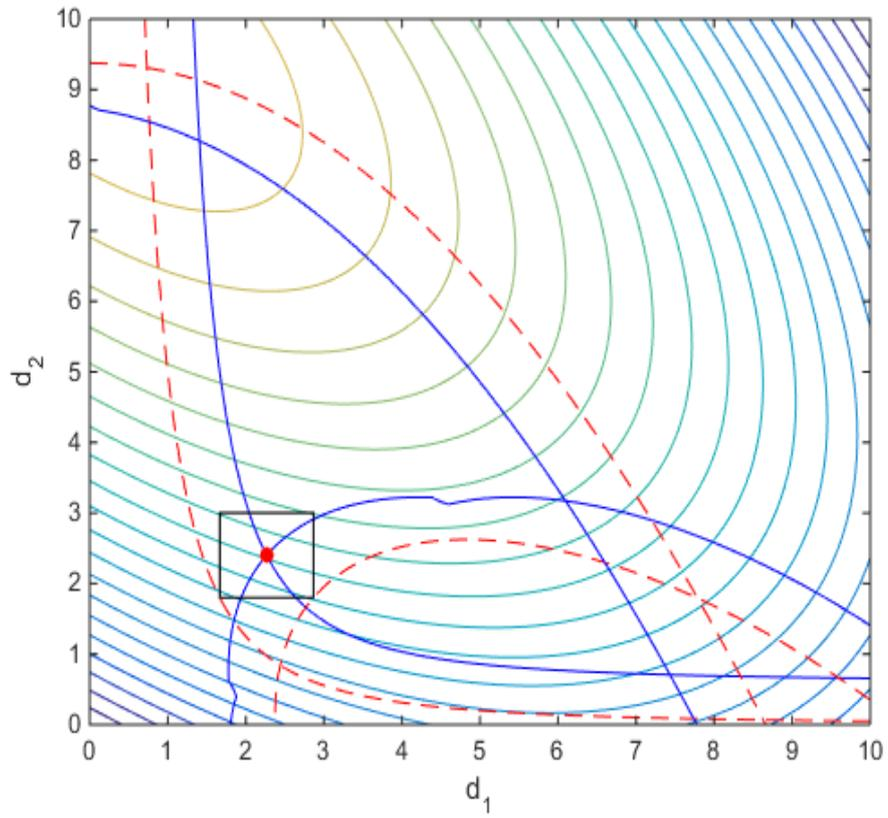
Fig. 1.29. Optimum and worst-case of constraints obtained by WWCO
