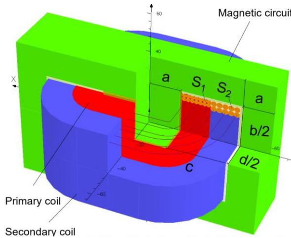
Fig. 3.9. The design variables of the transformer
