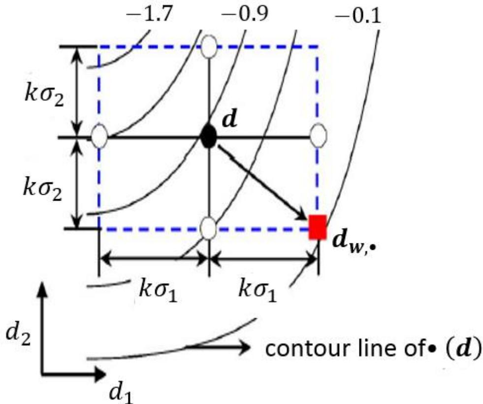
Fig. 1.6. Worst-Vertex-based WCO (Z. Ren et al., 2013)
