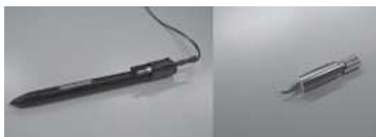
Figure 2.10 The stylus and the vibration motor (adapted from [54]).
