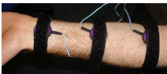
Figure 2.12 Putting three vibrators on the forearm to encode information (adapted from [59]).
