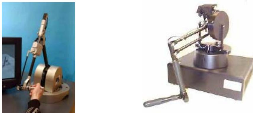
fig. 1-5: Le Virtuouse6D [http] et le PHANToM6D [http]
