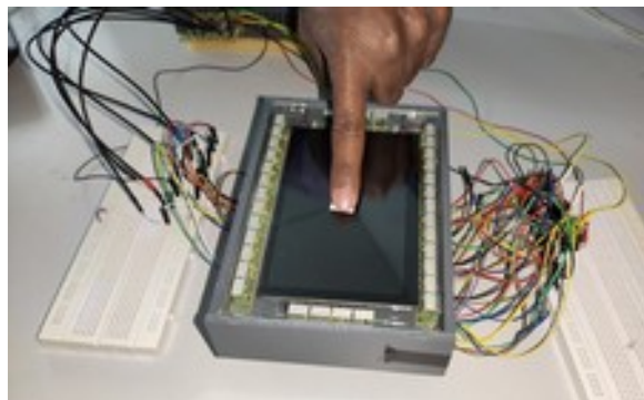
figure 1: An experimental Device at L2EP which can control the vibration of a plate in the middle with actuators placed at the periphery. The user feels like a button click with an appropriate control.
