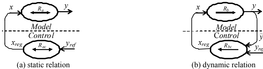
Figure B-8: COG of static and dynamic relations with their control schemes.
